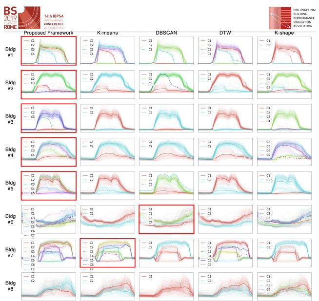
Figure 3: Clustering results of different methods on 8 exemplary buildings (best cases highlighted in red boxes).
