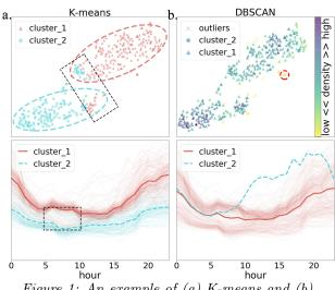
Figure 1: An example of (a) K-means and (b) DBSCAN giving bad clustering results (Upper: 2-D visualization; lower: time series load profile.)
